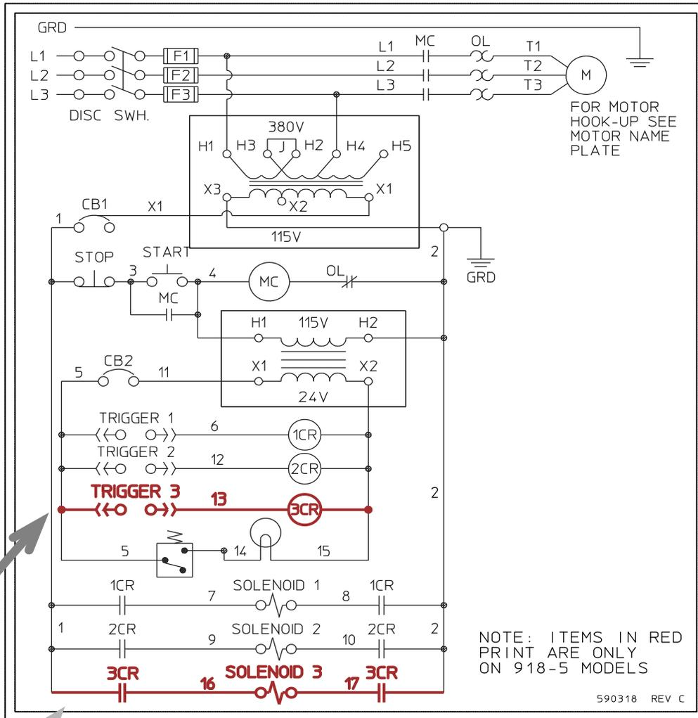
**NOTE: The graphics identified below appear in RED printing on the schematic.**
